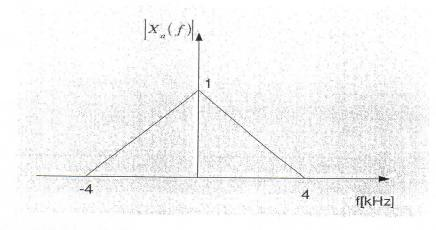
A discrete-time signal  $x_1(n)$  was generated by sampling the signal  $x_a(t)$  using the sampling frequency  $F_{sl} = 8 kHz$ .
